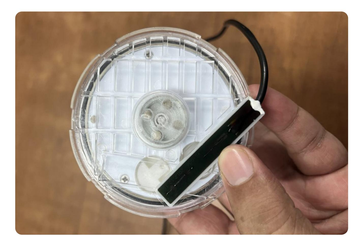
2. Sensor cable has 3 wire endings – Red (Positive input), Black (Negative input) & Light green/Yellow (Common) as shown in picture below. Connect them to the respective ports of a Pulse Counter / GSM/GPRS RTU.
