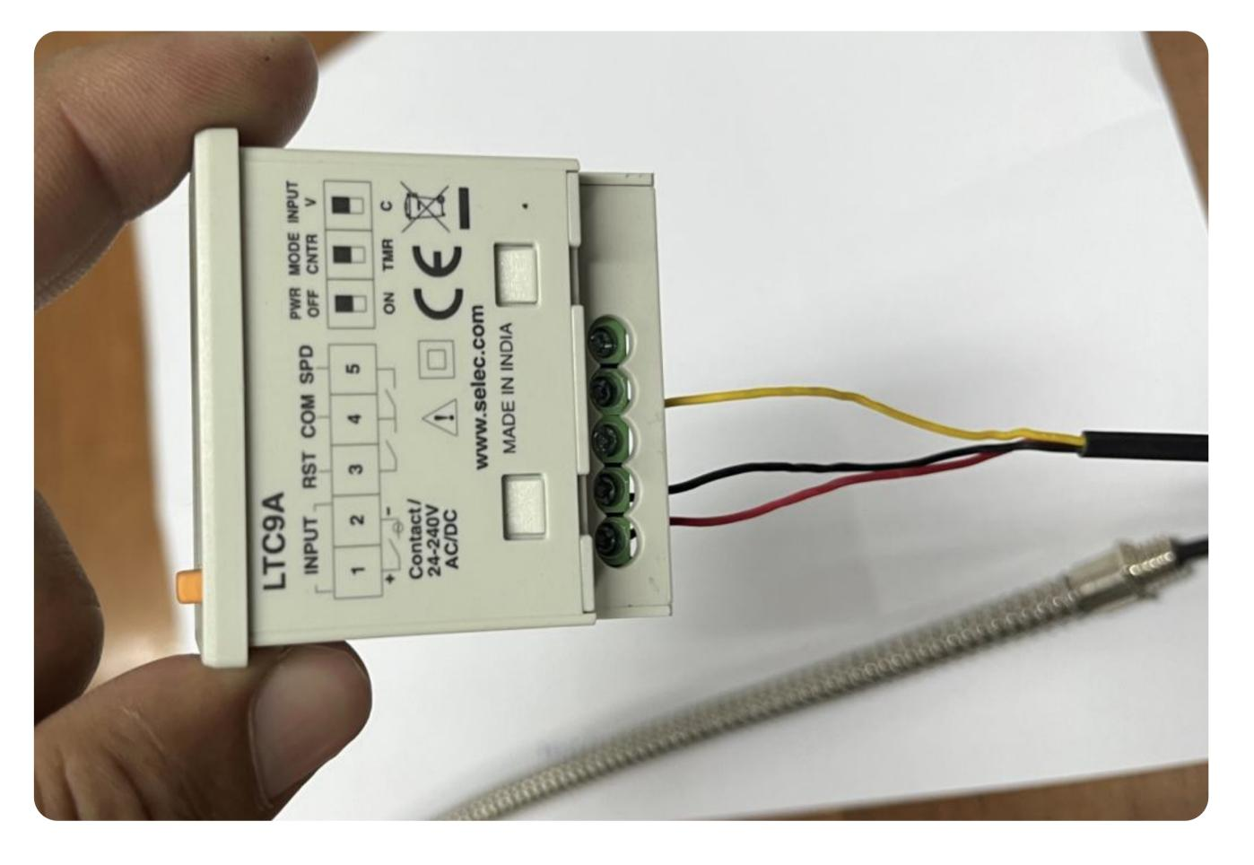
3. After all the correct connections, pulse counter will give one pulse output for each complete revolution of the pointer of respective ancillary scale.
